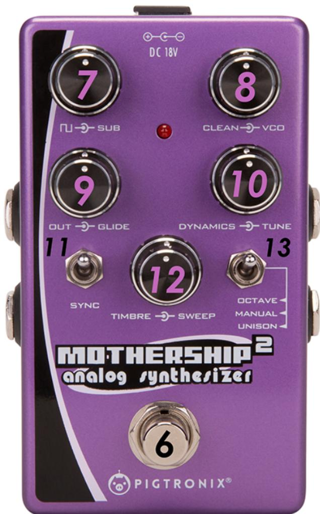
6. **ENGAGE** - This footswitch turns the entire Mothership 2 on and off. When the engage light is turned on, the Mothership 2 is active. The Mothership 2 is a true bypass pedal.
