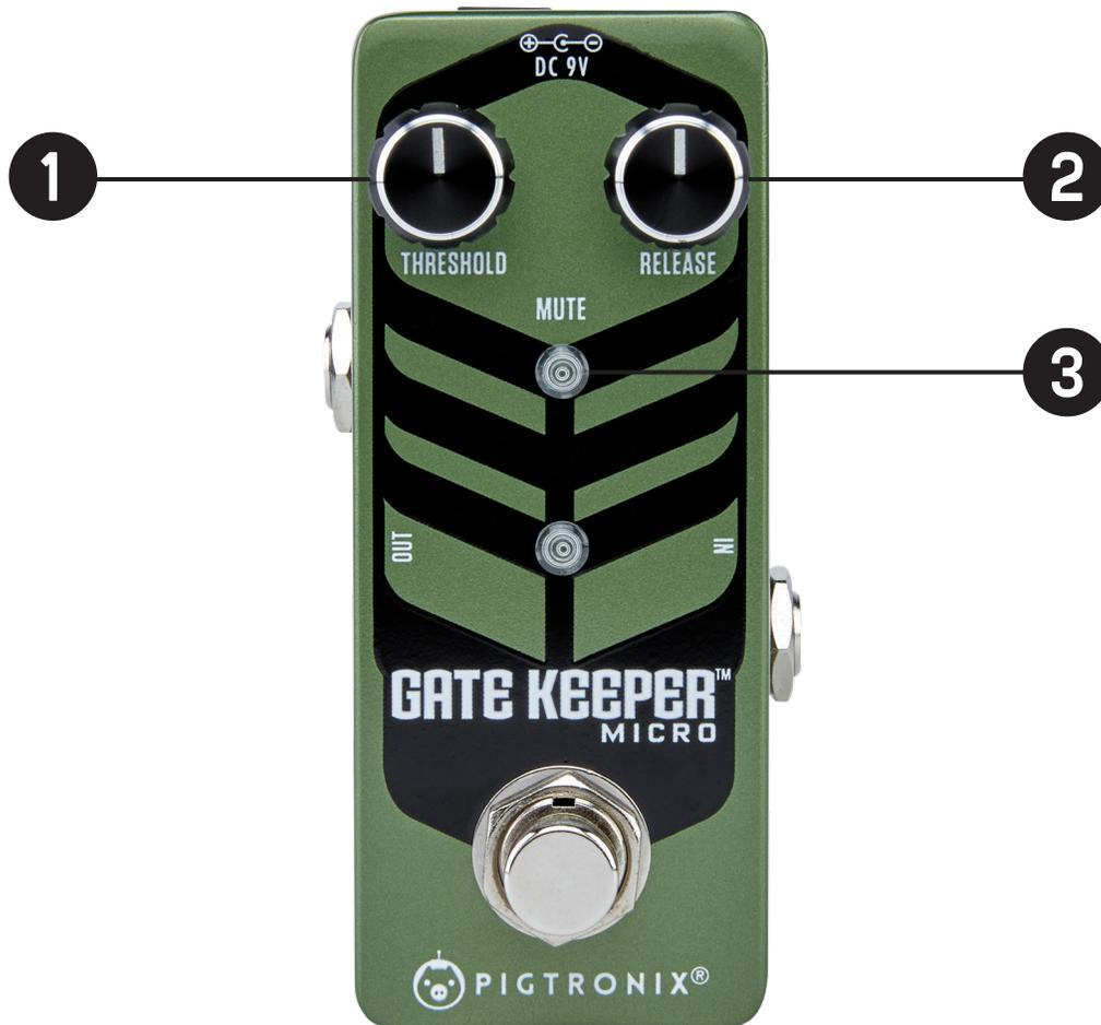
**1** **Threshold** is the most important control on the Gatekeeper pedal. This knob controls how much signal is needed in order to open the gate. The hotter the signal you put into the Gatekeeper, the lower the Threshold knob should be set.
